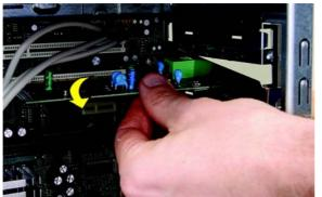
Figure 2-17 Rocking the card to Remove
